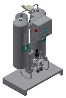
Pressure Swing Adsorption (PSA). This technology uses a molecular screen bed of desiccants known as Carbon Molecular Sieve, in order to effectively remove (extract) oxygen and carbon dioxide molecules from the compressed air. The two screens switch alternatively from the filter mode to regeneration mode to ensure a consistent supply of nitrogen.
