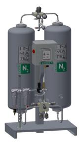
The technology associated with supplying a constant and purified Nitrogen Gas is referred to Pressure Swing Adsorption (PSA). This technology uses a molecular screen bed of desiccants known as Carbon Molecular Sieve, in order to effectively remove (extract) oxygen and carbon dioxide molecules from the compressed air. The two screens switch alternatively from the filter mode to regeneration mode to ensure a consistent supply of nitrogen.
