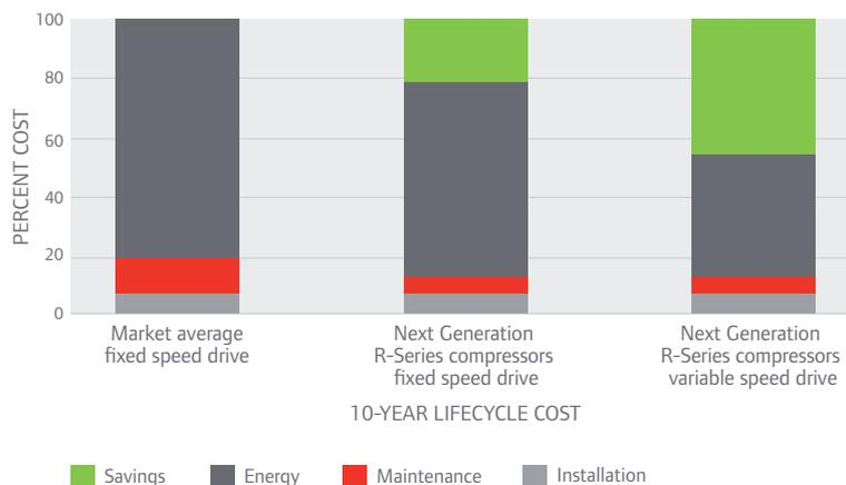
Rotary comparison at 79% average volume capacity; 4000 hours per year; 0.1€/kWh
