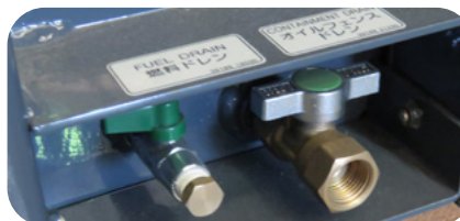
External fuel and oil drains for fast servicing
