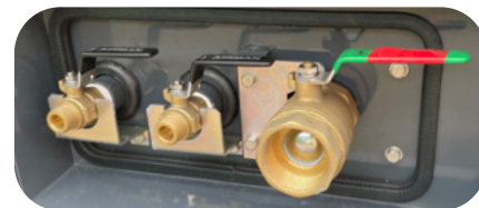
Large 2"x1"(F), 2x 3/4"(M) air outlets
