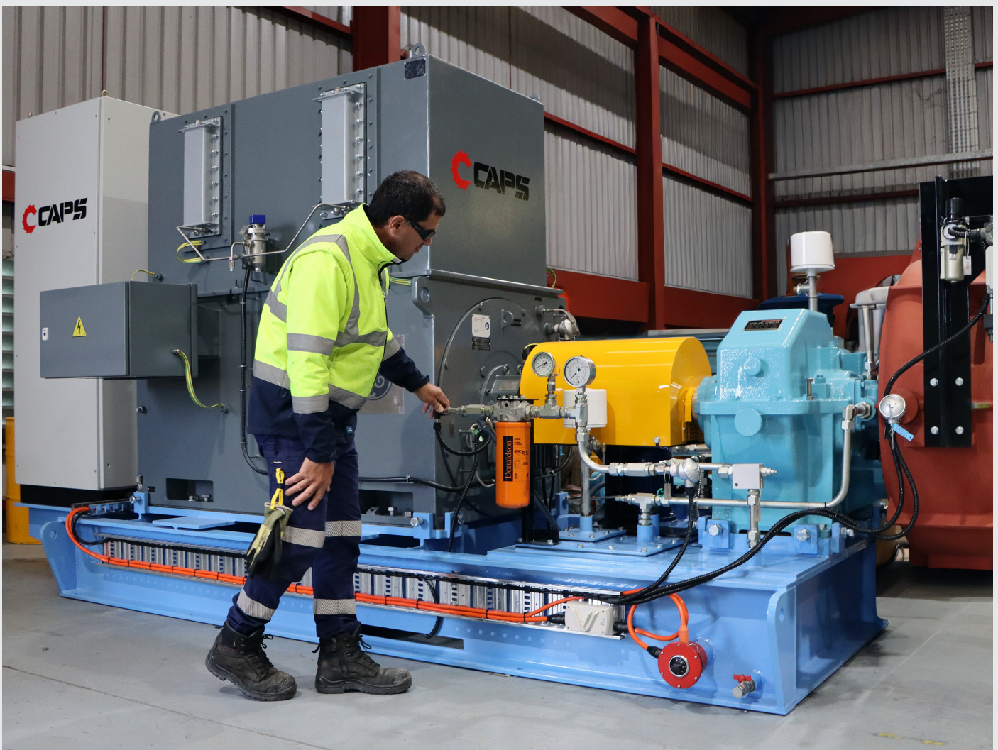
GM45H, CAPS KHI BLOWER, Single Stage Geared - 553 m 3 /min, 212 Kpa(A), 1100 Kw Manufactured & assembled at our CAPS Perth engineering facility.
